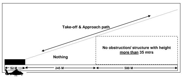
3.6 The site and adjoining area, up to a distance of 500 Metres from the centre of the helipad Site selected, should be free of electric wires, telephone cables, data/tv cables, microwave tower, transformers and any such objects that may become an obstruction for safe operation of the helicopter.
